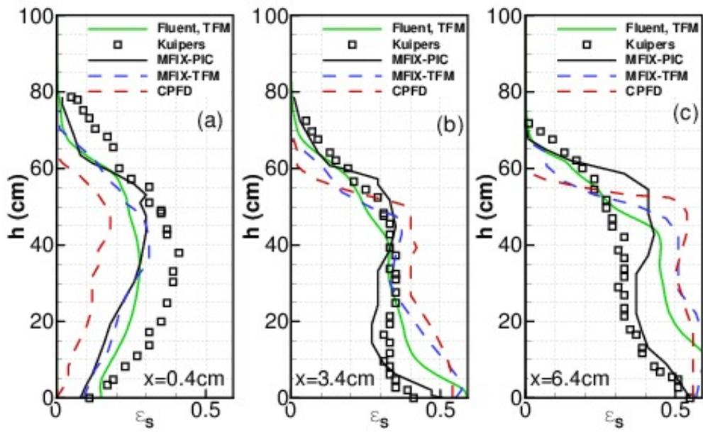
FIGURE 6. Average volume fraction (20–30sec) distribution of solid particles along 3 vertical lines at  $x=0.4\text{cm}$ (a),  $x=3.4\text{cm}$ (b),  $x=6.4\text{cm}$ (c) from the central jet.
