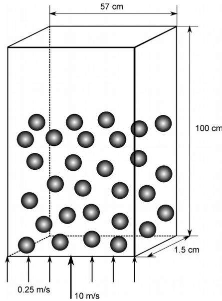
FIGURE 1. The fluidized bed test setup by Kuipers [4]
