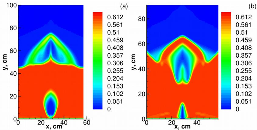
FIGURE 2. Bubble evolution at 1 sec (a) and 9 sec (b).
