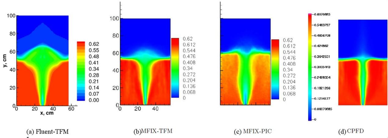
FIGURE 4. Time-averaged solid volume fraction of the present simulation (a) compared with literature data [7].
