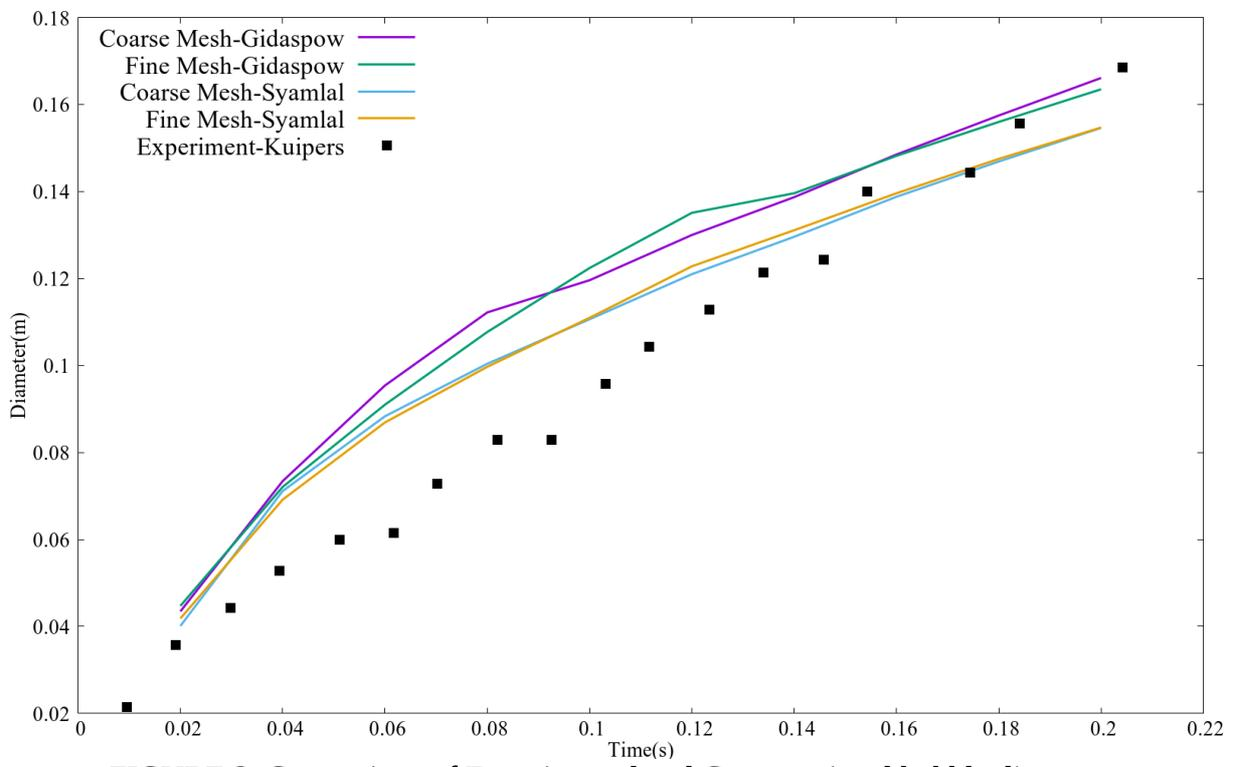
FIGURE 3. Comparison of Experimental and Computational bubble diameters
